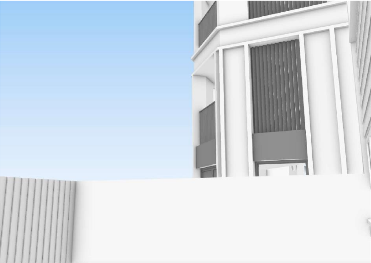
Image of window louvres deflecting views away from rear garden of No.2
